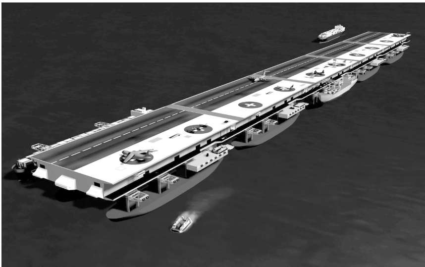
FIG. 8. — Illustration of Mobile Offshore Base concept (from McDermott Technology, Inc.; used with permission). The rubber connectors would be located between each of the five detachable modules.
