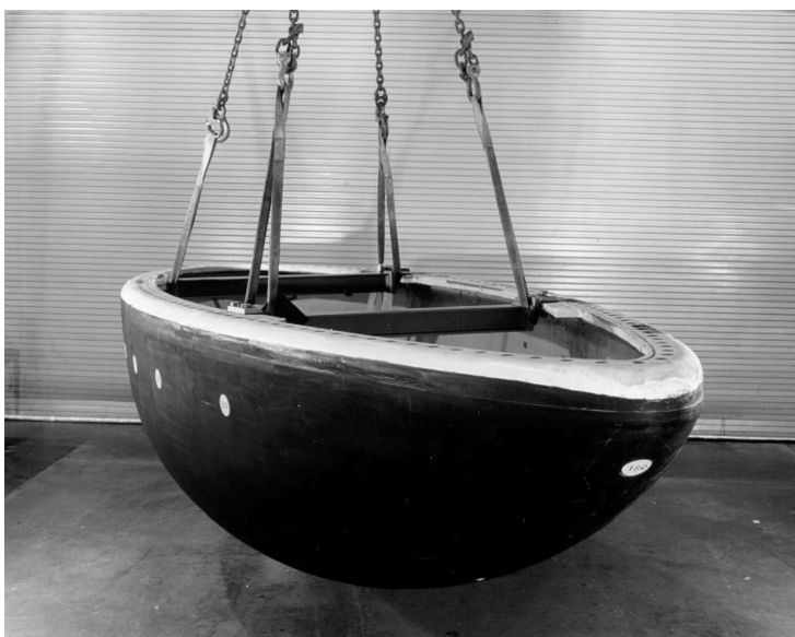
FIG. 4. — Composite rubber/reinforced plastic keel dome.
