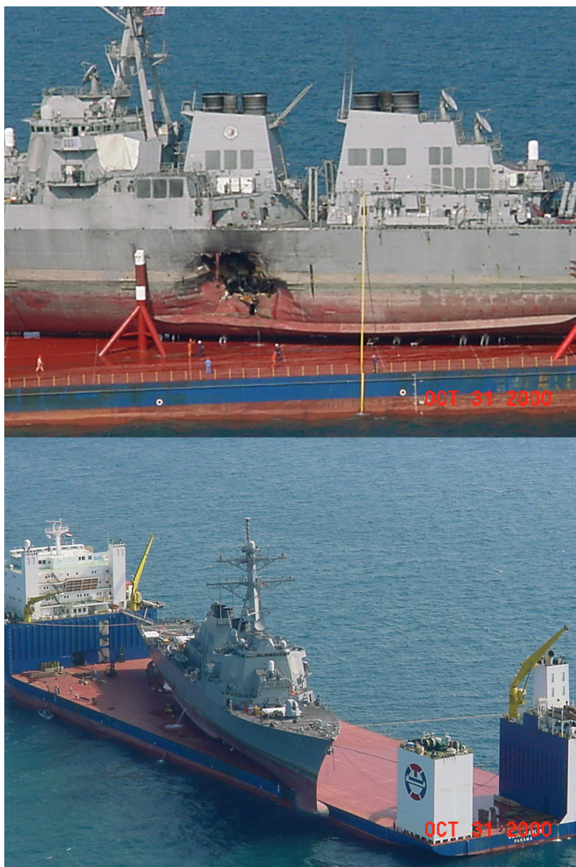
FIG. 2. — The guided missile destroyer USS Cole , being returned to the United States after the terrorist attack in Yemen. Despite the damage to the hull, as well as the severe jostling when mounted on a Norwegian transport vessel (top), the bow dome (seen in lower photograph, hanging off the edge of the transport) remained functional. After repairs that included replacement of 550 tons of exterior steel plating, the Cole returned to sea duty 18 months later.
