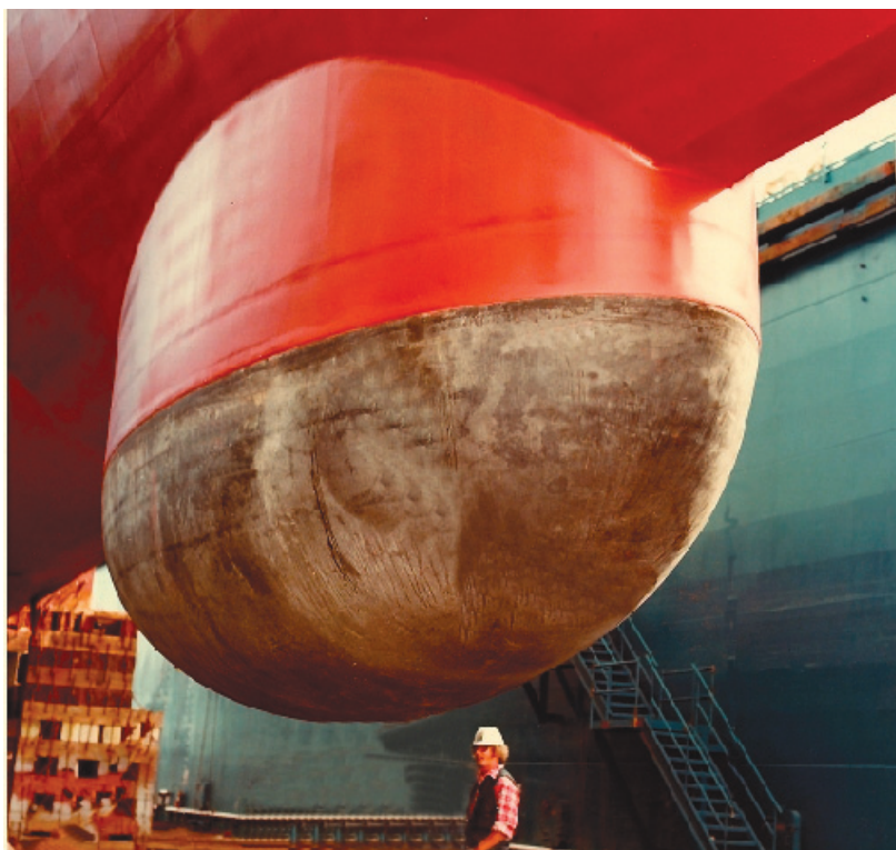
FIG. 3. — Rubber sonar dome mounted to bow of ship.
