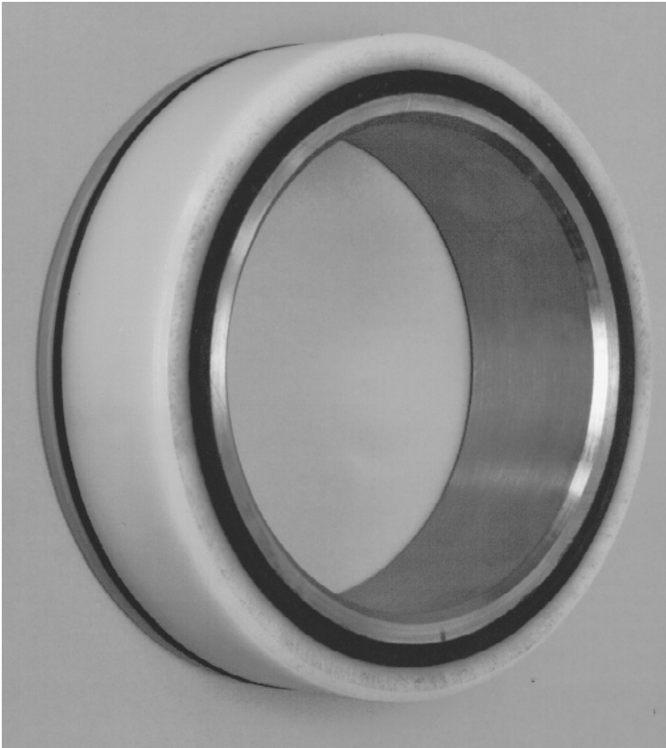
FIG. 5. — Thrust reducer to decouple the propeller from the submarine. The natural rubber is sandwiched between the steel ring and an outer layer of polyethylene.
