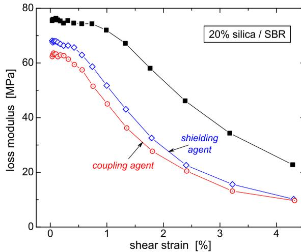
**Figure 1** Dynamic loss modulus as a function of shear strain for SBR reinforced with 20% by volume silica: untreated (squares); with 6.5% by weight *n*-octyltriethoxysilane shielding agent (diamonds); or 4.7% by weight 3-mercaptopropyltrimethoxysilane coupling agent (circles). Suppression of agglomeration reduces the hysteresis (Robertson *et al.*, 2011).
