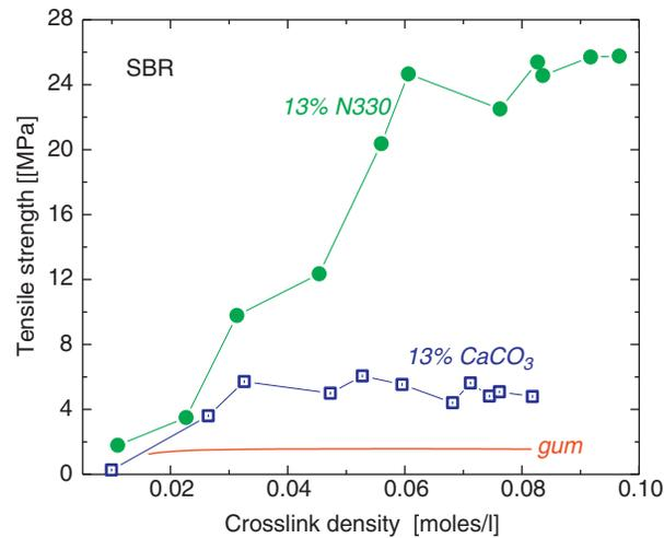
**Figure 7** Tensile strength of SBR unfilled (line), with 0.13 volume fraction (45 phr) calcium carbonate (squares), and with 0.13 volume fraction (30 phr) HAF carbon black, as a function of crosslink density (Bueche, 1958).
