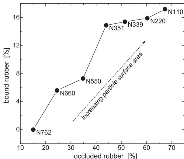
**Figure 4** Quantity of rubber bonded to the filler versus the amount of rubber occluded in the particle structure for a 1,4-polybutadiene with 18% by volume carbon black of the indicated type (Robertson *et al.*, 2007).
