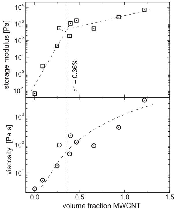
**Figure 3** (Lower) Viscosity of PTMO as a function of filler content; the fitted line is the Guth–Gold equation with  $f=21$ . (Upper) Storage modulus of the same compound, with the change in slope at a value of  $\phi$  for which the percolation equation (eqn [3]) gives  $f=16$  (Casalini *et al.*, 2012).
