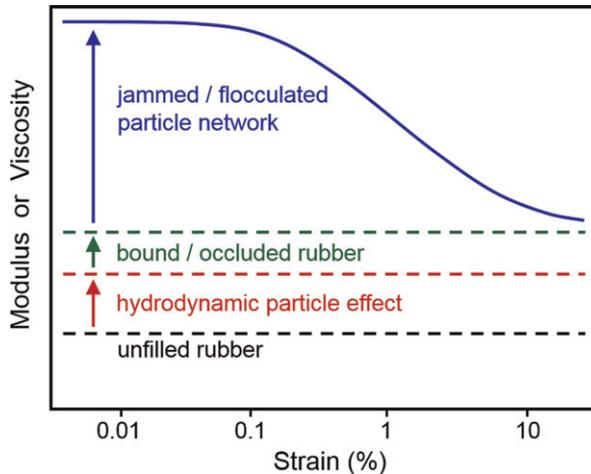
**Figure 2** Schematic depicting the various contributions to the modulus and viscosity of rubber.
