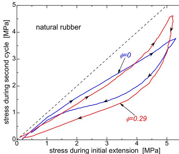
**Figure 6** Stress measured during extension–retraction of natural rubber unfilled (blue line) and containing 29% by volume (80 phr) N330 carbon black (red line). The abscissa is the stress for the first extension cycle and the ordinate is the stress for subsequent cycles. The dashed line corresponds to zero hysteresis (Roland, 2011).
