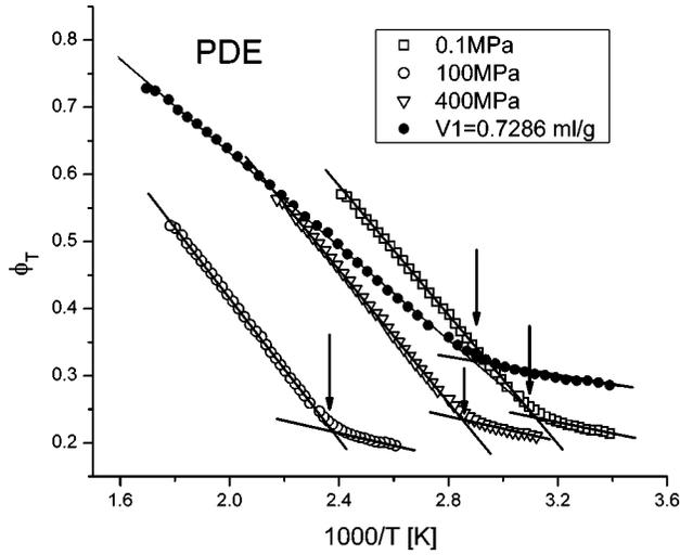
FIG. 2. Stickel function,  $\phi_T$ , for dielectric relaxation time of PDE. The lines indicate the respective low and high  $T$  linear fits, done over the range  $-2.27 < \log_{10}(\tau[\text{s}]) < 1.68$  and  $-8.76 < \log_{10}(\tau[\text{s}]) < -5.08$ , whose intersection defines the dynamic crossover [values of  $T_B$  and  $\log(\tau_B)$  listed in Table I].
