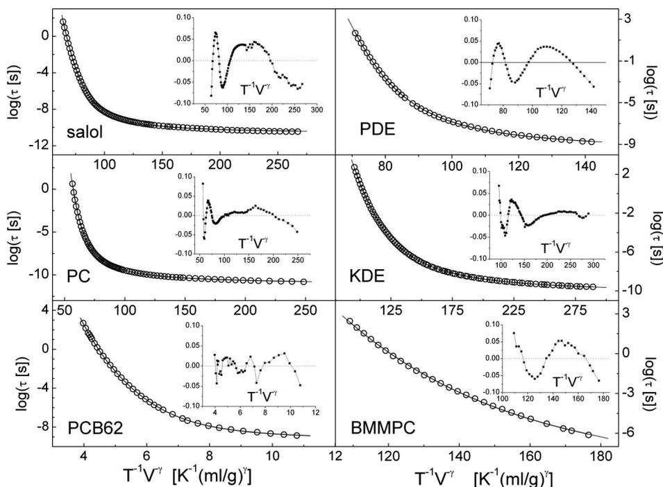
FIG. 12.  $\log(\tau)$  vs  $T^{-1}V^{-\gamma}$  for the six materials studied herein, along with the best fit of Eq. (10). The fit parameters are given in Table II. The residuals are plotted in the insets.
