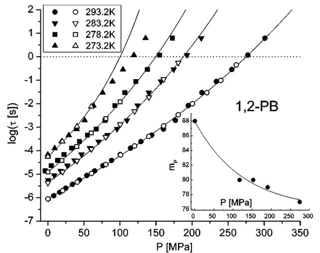
FIG. 11.  $\log(\tau)$  vs  $P$  for 1, 2-polybutadiene measured at four temperatures. Open symbols are experimental data, closed symbols were calculated from data at atmospheric pressure using  $\log(\tau)=\mathcal{J}(TV^{1.9})$ . Solid lines represent fits to Eq. (5). The inset shows the  $m_P$  calculated from the isotherms using  $\log(\tau)=\mathcal{J}(TV^{1.9})$ .
