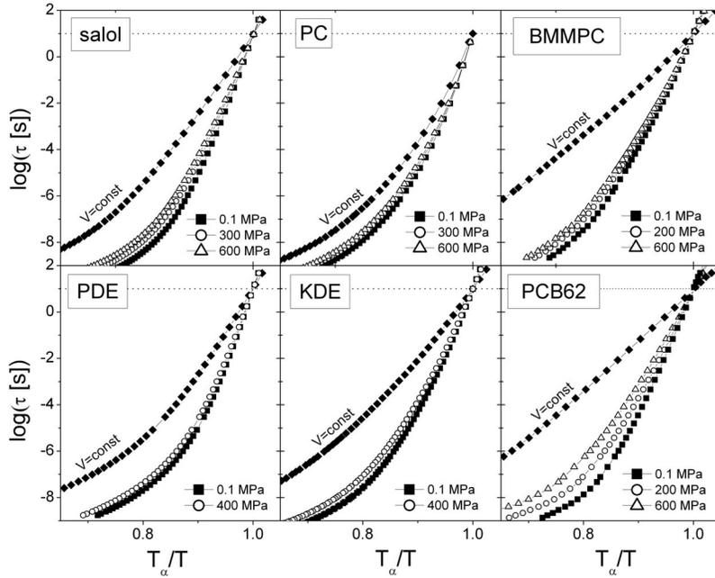
FIG. 9. Isobaric dielectric relaxation times for salol, PC, BMMPC, PDE, KDE, and PCB62 versus  $T_\alpha/T$  where  $\tau(T_\alpha)=10$  s. Isochors were calculated at the volume at which  $\tau=10$  s at atmospheric pressure;  $V=0.7907$  (salol),  $0.7558$  (PC),  $0.9067$  (BMMPC),  $0.7297$  (PDE),  $0.7748$  (KDE), and  $V=0.6131$  (PCB62) ml/g.
