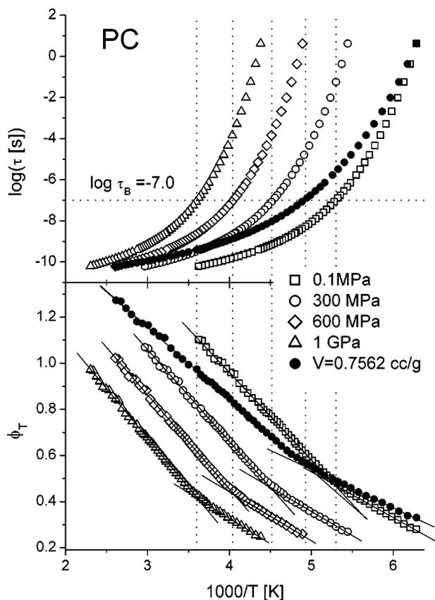
FIG. 4. Upper panel: dielectric relaxation time for PC (experimental data for 0.1 MPa; other isobars and isochoric curve were calculated). Dotted line indicates the average of  $\log(\tau_B)$  for the different curves. Lower panel: Stickel function, with low and high  $T$  linear fits, done over the range  $-6.14 < \log_{10}(\tau[s]) < 0.63$  and  $-10.21 < \log_{10}(\tau[s]) < -8.03$ , respectively. The vertical dotted lines in both panels represent the dynamic crossover (see Table I).
