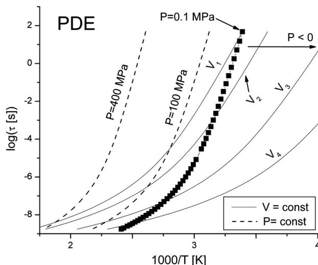
FIG. 1. Dielectric relaxation time for PDE. Solid lines are calculated isochoric curves for  $V_1=0.72865$ ,  $V_2=0.7380$ ,  $V_3=0.7602$ , and  $V_4=0.7795$  cm<sup>3</sup>/g. Dotted lines are calculated isobaric curves for  $P=100$  and  $400$  MPa. Points (■) are for atmospheric pressure.
