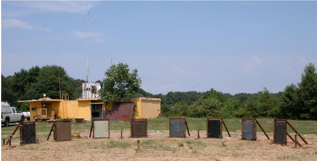
Fig. 4 — Typical arena blast test configuration, with test plates mounted in a semicircle, 0.94 m from the explosive. Interspersed between these test panels are four pressure transducers to measure the blast pressure incident on the targets.
