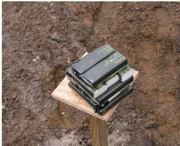
Fig. 5 — Blocks of C4 explosive arranged to give a symmetrical blast pressure at the targets
