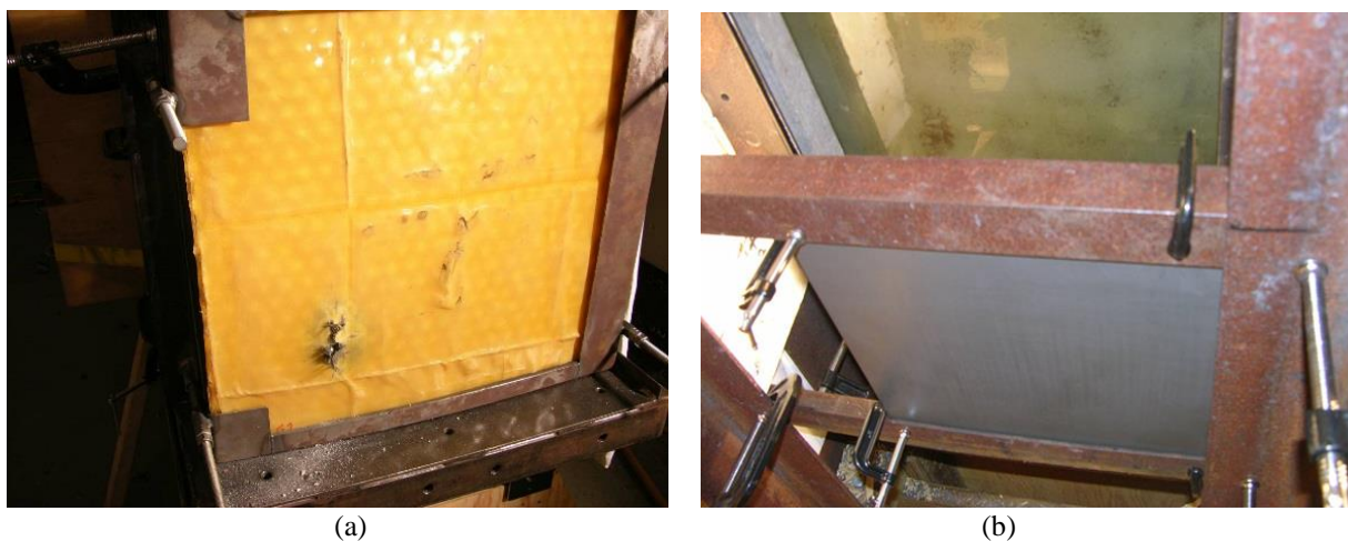
Fig. 3 — (a) Front side of target after penetration in lower left corner by three .50 caliber armor-piercing projectiles. (b) Intact witness plate demonstrating the absence of complete penetration of the target.
