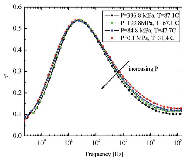
**Figure 11.** Dielectric loss peak in PMA at state points for which  $\tau_\alpha$  is constant. The ordinate values were normalized to superpose the peak. The spectra narrow with increasing pressure, with  $\beta_{KWW}$  in the range  $0.40 < \beta_{KWW} < 0.44$ .
