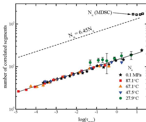
**Figure 7.**  $N_c$  and  $N_{\alpha}$  for PMA at atmospheric pressure and  $N_c$  at high pressure. The solid line is a linear fit to the  $N_c$  data; the dotted line is this fit after adjusting by the factor from eq 5.
