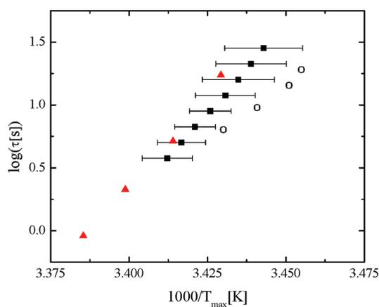
**Figure 5.** Relaxation times  $\tau$  ( $1/2\pi f_{\max}$ ) for PMA versus the inverse of the temperature of the peak maximum determined from the fit of a Gaussian to the peak in the isochronal dielectric loss (squares) and the peak in the MDSC  $C_p''(T)$  (circles). The relaxation times (circles) determined from the fit of eq 1 to the dielectric spectra measured in the frequency domain are also shown (see Figure 2).
