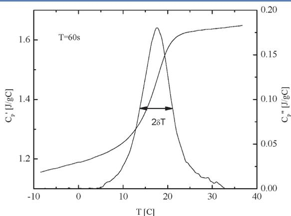
**Figure 4.** Real and imaginary parts of the heat capacity of PMA for a 60 s modulation period. Before calculating  $C_p''$ , the phase angle was corrected as discussed by Weyer et al.<sup>43,44</sup>
