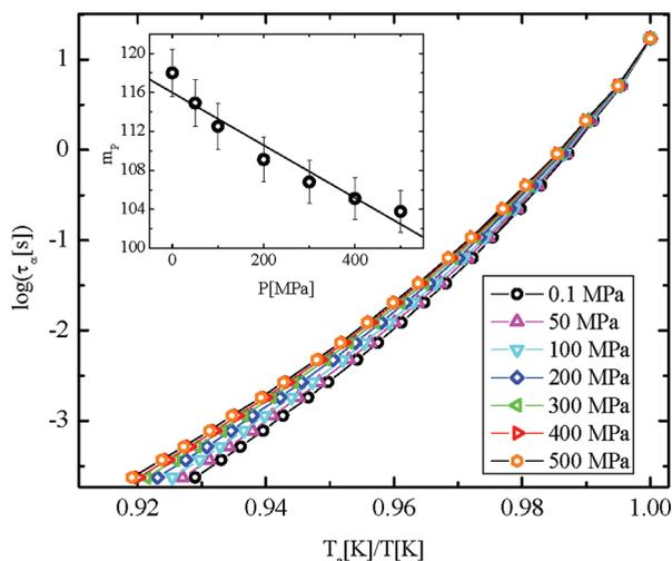
**Figure 12.** Segmental relaxation times of PMA versus  $T_a$ -normalized temperature for the indicated pressures. The steepness of the curves decreases with pressure (inset), with  $dm/dP = -27 \pm 5 \text{ GPa}^{-1}$  at ambient pressure as determined from the linear fit (solid line).
