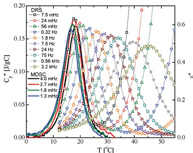
**Figure 6.** Isochronal response of PMA measured by MDSC (solid lines) and dielectrically (symbols with dotted lines) at the indicated frequencies. For a given frequency, the calorimetry peak is at higher temperature. Note the rise in  $\epsilon''(T)$  at lower  $T$  due to the increasing contribution of the  $\gamma$  process.
