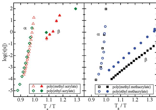
**Figure 13.**  $\alpha$ - (open symbols) and  $\beta$ - (solid symbols) relaxation times for PMA, PMMA, PEA and PEMA versus the inverse temperature normalized to the glass temperature. The  $\beta$  process for the acrylate polymers is several orders of magnitude closer to the  $\alpha$  process than in the poly(methyl acrylate)s. Data for PMMA from ref 61 and for PEA and PEMA from ref 62.
