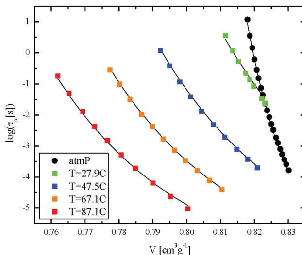
**Figure 8.** Dependence of the segmental relaxation time of PMA on the specific volume at atmospheric pressure and for four isotherms ( $291.6 \text{ K} < T < 313.9 \text{ K}$ ). The solid lines represent the fit of the scaling function derived from the Avramov model (eq 9).
