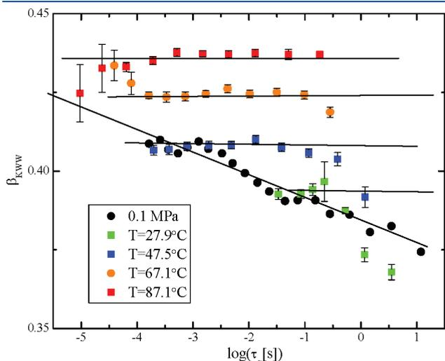
**Figure 3.** Kohlrausch exponent for the  $\alpha$  process in PMA versus  $\log(\tau_\alpha)$  at atmospheric pressure for four isotherms ( $291.6 \text{ K} < T < 313.9 \text{ K}$ ). The lines are to guide the eye.
