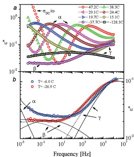
**Figure 1.** (a) Dielectric loss of PMA at atmospheric pressure and various temperatures. The  $\beta$  process is obscured by other, more intense relaxation peaks. (b) Dielectric loss of PMA at atmospheric pressure and two temperatures below  $T_g$ . The weak  $\beta$  process is indicated. The contribution of the three relaxations are shown by the fitted curves (dotted lines for  $-26.9$  °C and solid lines for  $-6.0$  °C).
