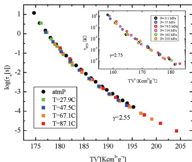
**Figure 9.** Scaling plot of the segmental relaxation time of PMA, with  $\gamma = 2.55$ . The inset is the scaling plot for the relaxation time measured using photon correlation spectroscopy,  $\tau_{PCS}$ , by Fytas et al.<sup>53</sup> with the value of  $\gamma$  indicated.
