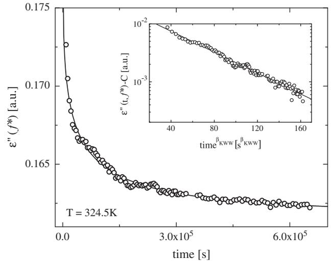
**Fig. 6.** Evolution during dielectric loss at  $f^* = 113$  Hz during aging at the indicated temperature. The solid line is the fit of Eq. (4) with constant  $\beta_{aging} = 0.38$ . The inset shows the same data after subtracting the fitting parameter  $C$ , plotted versus  $t^{\beta_{aging}}$ , with the line representing a linear fit.
