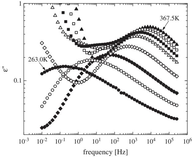
**Fig. 1.** Dielectric loss spectra for PMMA; from left to right the temperatures are 263.0, 290.5, 312.6, 338.2, 351.5, 357.4, 362.6, and 367.5 K. At higher  $T$  a strong  $\sigma_{DC}$  conductivity is evident.
