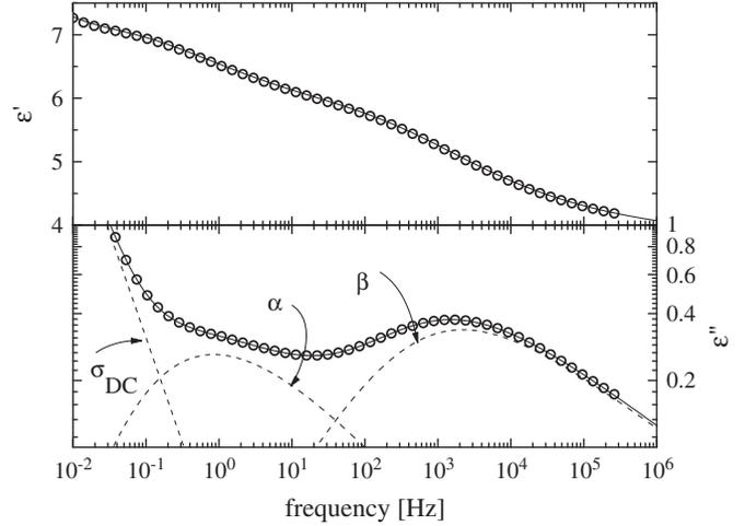
**Fig. 2.** Dielectric constant (top) and loss (bottom) of PMMA at 351.5 K. The solid lines are the fit of Eq. (1), with the dotted curves representing the respective contributions of the DC conductivity and the  $\alpha$  and  $\beta$  relaxations.
