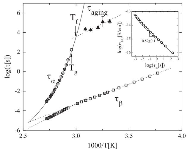
**Fig. 3.** Arrhenius plot of  $\tau_\alpha$ ,  $\tau_\beta$ , and  $\tau_{aging}$ , the latter from fitting Eq. (4). The inset shows a double logarithmic plot of the conductivity versus the  $\alpha$  relaxation time, yielding the indicated value of  $p$ .
