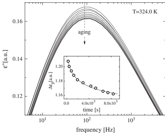
**Fig. 5.** Dielectric  $\beta$  loss peak of PMMA during aging at 324.0 K. The aging times were from  $2.6 \times 10^4$  to  $8.4 \times 10^5$  s (top to bottom). The inset shows the corresponding changes in the dielectric strength of the  $\beta$  peak during aging; the line is a stretched exponential with  $\beta_{KWW} = 0.38$  and  $\tau_{aging} = 2.2 \times 10^4$  s.
