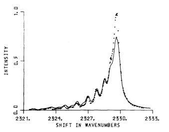
FIG. 8. The crosses show the experimental CARS Q branch of N<sub>2</sub> at a density of 2.5 amagat( $\simeq 40$  psia) and room temperature. The solid curve is a calculated spectrum fitted to the experiment using the same parameters (Q branch splitting, intensity ratio, and laser linewidths) as in Fig. 7, except that the collision-broadened intrinsic width of the Q branch lines was adjusted to give the best fit to the spectrum at large J (i.e., in the region 2325-329 cm<sup>-1</sup>).
