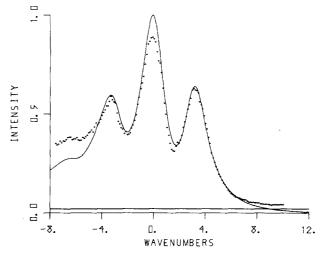
FIG. 5. The same band as shown in Fig. 4, but for a solution which is 67% CCl<sub>4</sub> by volume in acetone. The main difference in the two is that the nonresonant background is larger here relative to the resonant signal than in Fig. 4. The horizontal line indicates the intensity due to  $B^2$ .
