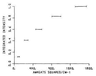
FIG. 12. A plot of the integrated intensity of the CARS Q branch spectra for N<sub>2</sub> as a function of the density squared over the bandwidth. If these bands are Lorentzian and if there are no extraneous sources of intensity, the points should fall on a straight line passing through the origin. Even when reasonable estimates of the uncertainty in the band width are included, the experimental results do not conform to this prediction.
