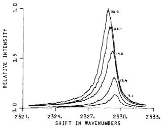
FIG. 10. Experimental measurements of the unresolved CARS Q branch spectra of  $N_2$  at several values of the density (indicated next to the appropriate curve, in amagat units). The intensity of the curve for the highest density was normalized to unity at the peak; other intensities are plotted relative to that value. The rapid increase in intensity is primarily a consequence of the dependence of CARS intensity upon the square of the density.
