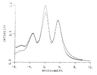
FIG. 4. The experimental CARS spectrum for the  $\nu_1$  of pure liquid CCl<sub>4</sub> is shown by the crosses. The three peaks are due to the three major isotopic species and the solid curve shows a calculated spectrum. The intensity due to  $B^2$  is neglibible on this scale. *B* is the (imaginary) nonresonant susceptibility.
