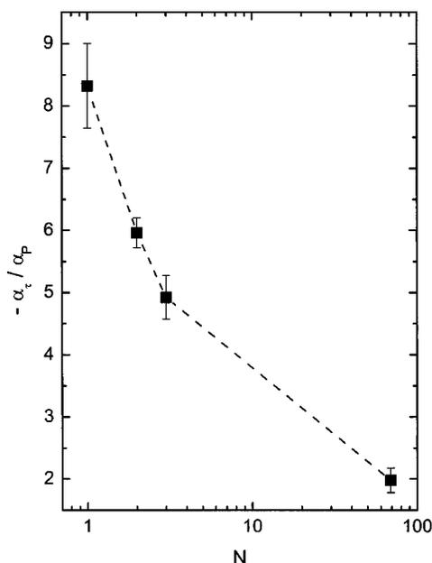
FIG. 9. Ratio of the isochronic ( $\tau=10^{-2}$  s) and isobaric ( $P=0.1$  MPa) thermal expansion coefficients ( $\blacksquare$ ) as a function of the degree of polymerization of the PPG.
