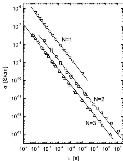
FIG. 3. Conductivity vs  $\alpha$ -relaxation time for propylene glycol ( $\nabla$ ) at  $T = 216.7$  K and  $65 < P$  (MPa)  $< 865$ , PPG dimer ( $\square$ ) at  $T = 216.8$ ,  $225.6$ , and  $238.4$  K and  $0.1 < P$  (MPa)  $< 594$ , and PPG trimer ( $\triangle$ ) at  $T = 223.5$ ,  $235.4$ , and  $245.3$  K and  $0.1 < P$  (MPa)  $< 632$ . The power-law fits to the data (solid lines) give  $k = 0.84 \pm 0.02$ .
