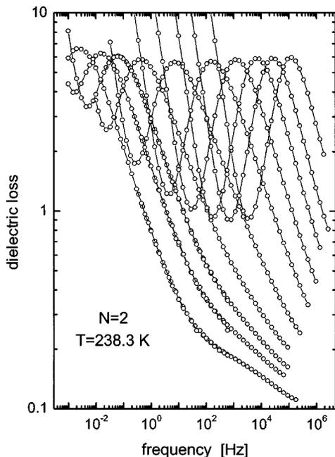
FIG. 1. Dielectric loss spectra for PG dimer at 238.3 K and (from right to left)  $P=0.1, 75.2, 140.9, 225.6, 319.7, 427.3, 512.2, 561.1, 593.5,$  and  $634.4$  MPa. The dc conductivity can be observed on the low frequency side of the  $\alpha$ -dispersion.
