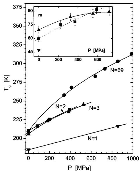
FIG. 4. Pressure dependence of the temperature at which the  $\alpha$ -relaxation time equals 0.01 s for PPG having the indicated degree of polymerization. The inset shows the pressure dependence of the fragility calculated from Eq. (4) for the dimer ( $\blacksquare$ ) and trimer ( $\blacktriangle$ ), along with the ambient pressure value for PG ( $\blacktriangledown$ ).
