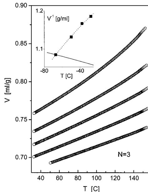
FIG. 7. The specific volume measured at pressures equal to (from top to bottom) 10, 30, 50, 90, 140, and 200 MPa for PPG trimer. The inset shows the variation of the density measured isochronally at  $\tau=0.01$  s (■) and isobarically at  $P=0.1$  MPa (solid line), from which the ratios in Fig. 5 were calculated.
