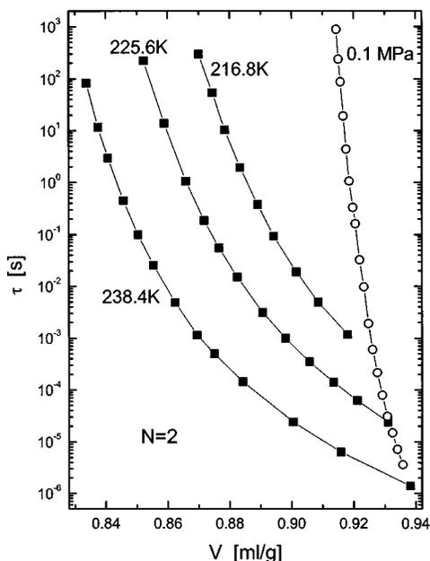
FIG. 8. The variation of the dielectric  $\alpha$ -relaxation times of the PPG dimer with specific volume, for measurements as a function of temperature at ambient pressure ( $\circ$ ) and as a function of pressure at the indicated temperatures ( $\blacksquare$ ).
