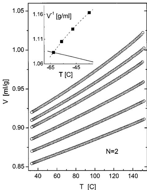
FIG. 6. The specific volume measured at pressures equal to (from top to bottom) 10, 30, 50, 90, 140, and 200 MPa for PPG dimer. The inset shows the variation of the density measured isochronally at  $\tau=0.01$  s (■) and isobarically at  $P=0.1$  MPa (solid line), from which the ratios in Fig. 5 were calculated.
