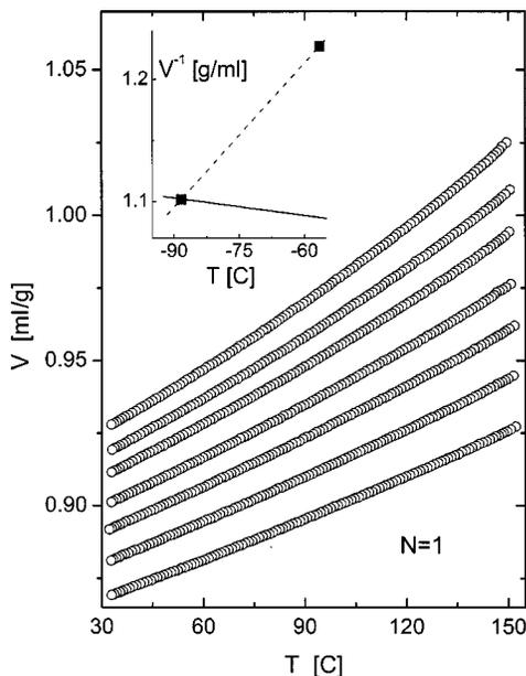
FIG. 5. The specific volume measured at pressures equal to (from top to bottom) 10, 30, 50, 80, 110, 150, and 200 MPa for PG. The inset shows the variation of the density measured isochronally at  $\tau=0.01$  s (■) and isobarically at  $P=0.1$  MPa (solid line), from which the ratios in Fig. 5 were calculated.
