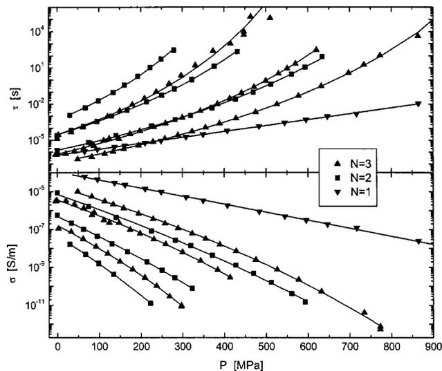
FIG. 2. Pressure dependence of the  $\alpha$ -relaxation times (upper panel) and conductivity (lower panel) for PPG dimer (■) at 216.8, 225.6, and 238.4 K, and trimer (▲) at 223.5, 235.4, and 245.3 K. Also shown are  $\tau$  for the monomer (▼) at 216.7 K. The solid lines are fits to Eq. (1).
