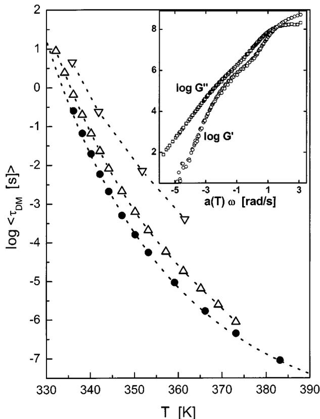
FIG. 8. Dynamic mechanical relaxation times versus temperature at  $P = 0.1$  MPa (●), along with the corresponding values from dielectric spectroscopy ( $\Delta$ ) and dynamic light scattering ( $\nabla$ ). The inset shows a master curve of the dynamic storage and loss moduli, for which the time-temperature shift factors,  $a(T)$ , were determined empirically, with  $a(T = 340 \text{ K})$  equal to unity.
