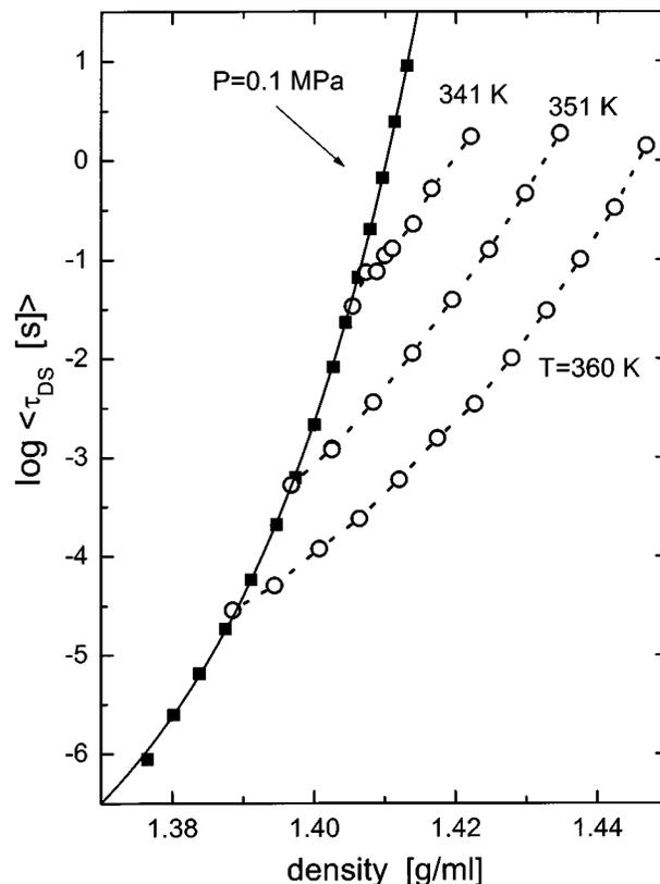
FIG. 9. The variation of the dielectric relaxation times with mass density, for measurements at varying temperatures and ambient pressure (■) and for varying pressures at the indicated temperatures in Kelvin (○). The density at  $T_g$  and atmospheric pressure was 1.41 g/ml.
