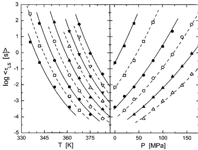
FIG. 7. Mean relaxation times measured by dynamic light scattering for isobaric conditions (from left to right, 0.1, 10, 20, 40, 60, 80, 100, 120, and 140 MPa) and isothermal conditions (341.2, 352.2, 361.2, 368.2, 375.2, and 383.2 K).
