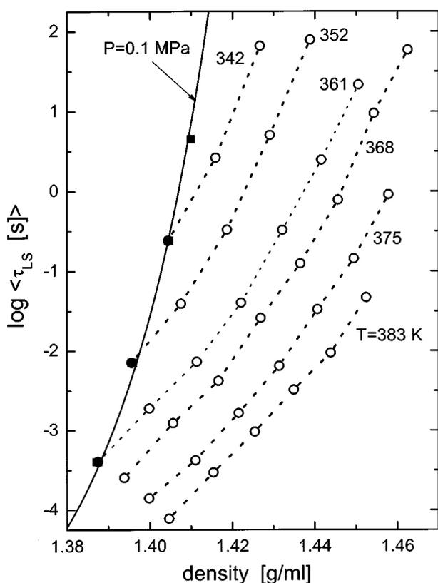
FIG. 10. The variation of the dynamic light scattering relaxation times with mass density, for measurements at varying temperatures and ambient pressure (■) and for varying pressures at the indicated temperatures in Kelvin (○). The density at  $T_g$  and atmospheric pressure was 1.41 g/ml.
