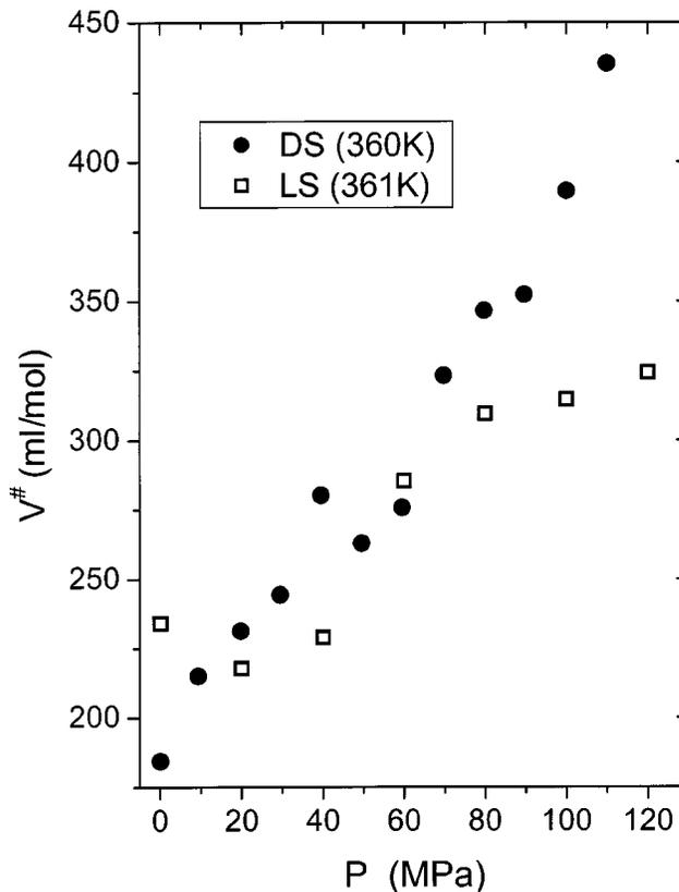
FIG. 13. Activation volume calculated from the pressure dependence of  $\langle \tau_{DS} \rangle$  (solid symbols) and  $\langle \tau_{LS} \rangle$  (hollow symbols) at approximately the same temperature.
