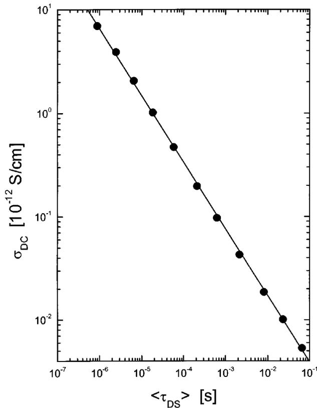
FIG. 5. Double logarithmic plot of the ionic conductivity versus the dielectric relaxation times for the atmospheric pressure measurements. We obtain for the exponent  $k = 0.645 \pm 0.004$  [Eq. (6)].
