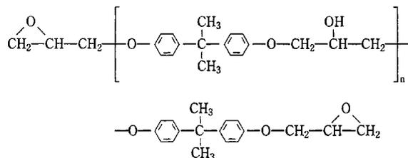
FIG. 1. The chemical structure of DGEBA ( $n=5$  herein).
