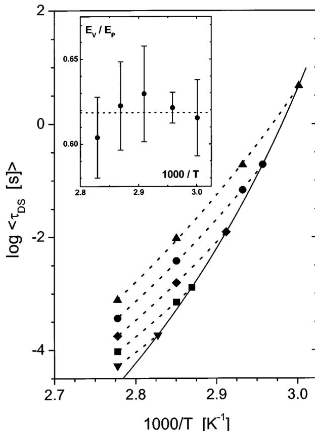
FIG. 11. Dielectric relaxation times calculated for a constant volume (dotted lines) equal to 0.01 (▲), 0.0125 (●), 0.015 (◆), 0.0175 (■), and 0.02 (▼) ml/g, and at constant pressure (solid line). The inset shows the ratio of the activation energy at constant volume to the enthalpy change at constant pressure. The mean value, =0.62, is indicated by the dotted line.
