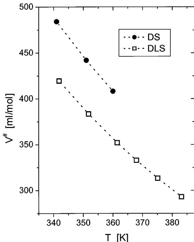
FIG. 14. Activation volumes, calculated from Avramov model using the parameters listed in Table I, at the indicated temperatures and corresponding pressures for which  $\langle \tau \rangle = 10$  s.
