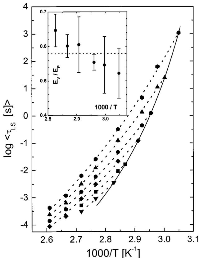
FIG. 12. Dynamic light scattering relaxation times calculated for a constant volume (dotted lines) equal to 0.0075 (hexagon), 0.01 ( $\blacktriangle$ ), 0.0125 ( $\bullet$ ), 0.015 ( $\blacklozenge$ ), 0.0175 ( $\blacksquare$ ), and 0.02 ( $\blacktriangledown$ ) ml/g, and at constant pressure (solid line). The inset shows the ratio of the activation energy at constant volume to the enthalpy change at constant pressure, with the mean value, =0.58, indicated by the dotted line.
