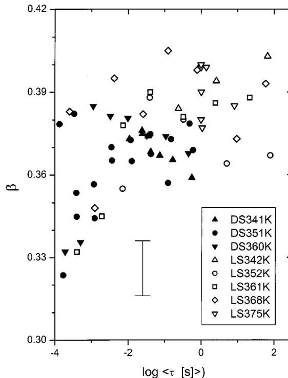
FIG. 4. Stretch exponents determined for the DS (solid symbols) and LS (hollow symbols) relaxation functions [Eqs. (4) and (12), respectively]. The uncertainty is as indicated.
