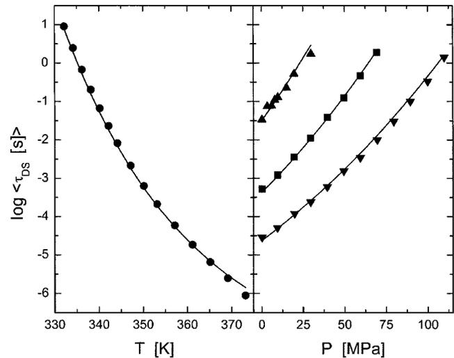
FIG. 6. Mean relaxation times measured by dielectric spectroscopy for isobaric conditions (at ambient pressure) and for isothermal conditions ( $T = 341.0, 350.8, \text{ and } 360.0 \text{ K}$ ).
