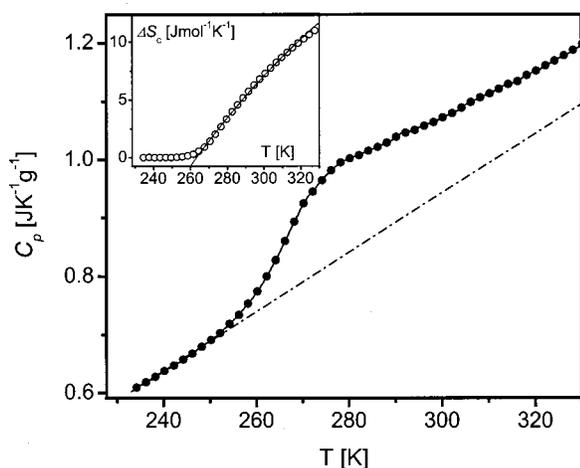
FIG. 7. Heat capacity for PCB62 measured during cooling at  $10 \text{ K min}^{-1}$ . The dashed line indicates a linear extrapolation of  $C_p^{\text{glass}}$  for  $T > T_g$ . The inset shows the entropy of the melt over that of the glass,  $\Delta S_c$  ( $\circ$ ), calculated as discussed in the text. The solid line is the fit for  $T > T_g$  of the function  $\Delta S_c = S_1 - k_1/T$ .
