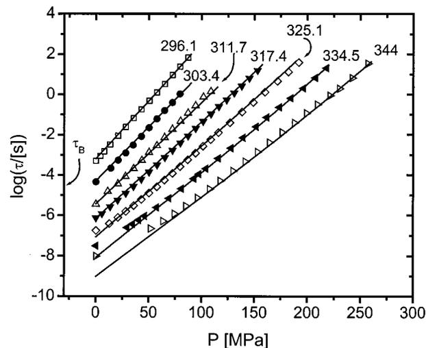
FIG. 5. Structural relaxation time of PCB62 vs pressure for seven temperatures (indicated in K in the figure). The solid line is the best fit of the data to a VF equation with  $T_0$  substituted by the function  $T_0^*(T,P)$  [Eq. (4)]. Note that the fit was carried out only for  $\tau > \tau_B$ , although we show the calculated curve for shorter  $\tau$  to emphasize the deviation at lower pressure for the higher temperatures.
