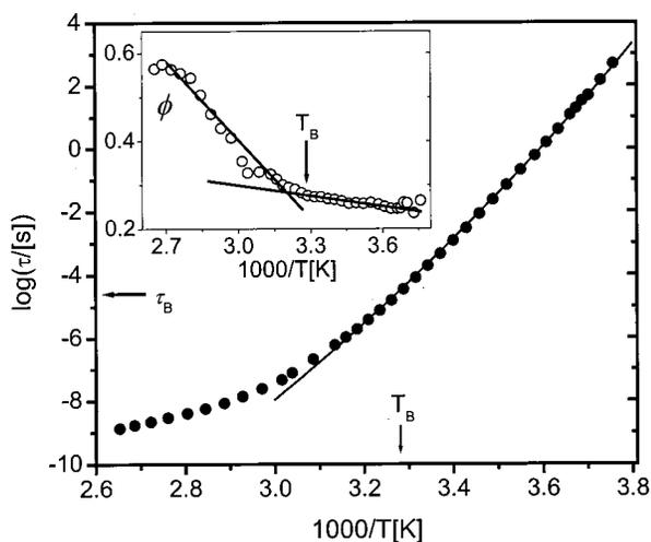
FIG. 4. Structural relaxation time of PCB62 measured at atmospheric pressure. The solid line is the best fit obtained by fitting the data to the VF equation with  $T_0$  substituted by the function  $T_0^*(T,P)$  [Eq. (4)]. The inset shows the Stickel function  $\phi = (d \log(\tau)/d(1000/T))^{-1/2}$ . The solid lines serve to emphasize the change of dynamics at  $T_B$  from the VF behavior observed for  $T_g < T < T_B$ .
