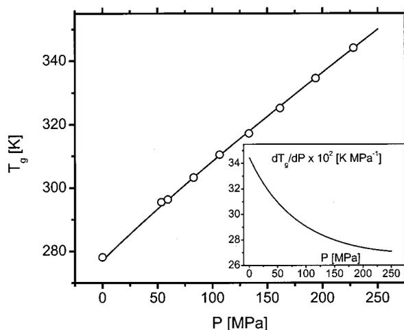
FIG. 6. Pressure dependence of the glass transition temperature  $T_g(P)$ , taken here as the temperature for which  $f_{\max} = 10^{-1}$  Hz (so that no extrapolation was necessary). The points are from the measured relaxation times, while the solid line is calculated from the AG model [Eq. (4)], using parameters estimated from the fit of the  $\tau(T, P)$  data. The inset shows the derivative of the latter.
