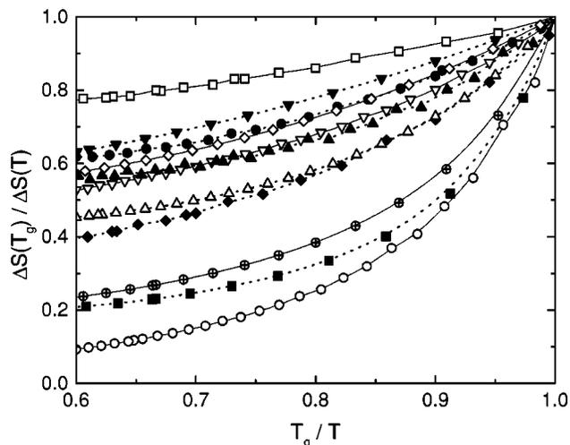
FIG. 6. The data in Fig. 4 replotted in a fashion analogous to dynamic fragility curves. The symbols are identified in Fig. 4.
