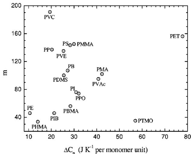
FIG. 2. Fragility versus the heat capacity change at  $T_g$  per mole of monomer units for 17 polymers (data from Table I), demonstrating the absence of any correlation between these quantities.
