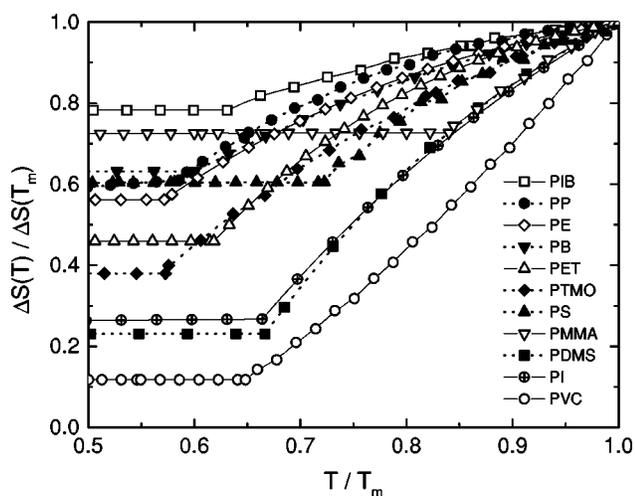
FIG. 4. Kauzmann plots for 11 polymers (see Table II). The steepness reflects the thermodynamic fragility (Ref. 8).
