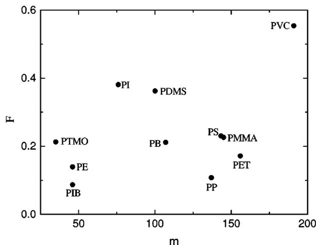
FIG. 5. Thermodynamic fragility, calculated from the data in Fig. 4 using Eq. (4), versus dynamic fragility.
