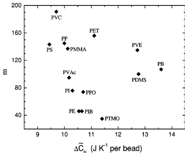
FIG. 3. Fragility versus the heat capacity increment at  $T_g$  per bead. This corresponds to Fig. 2 with the abscissa divided by  $n$ . These normalized heat capacity values fall within a narrow range (Refs. 31,33,34) while the fragility is widely scattered.
