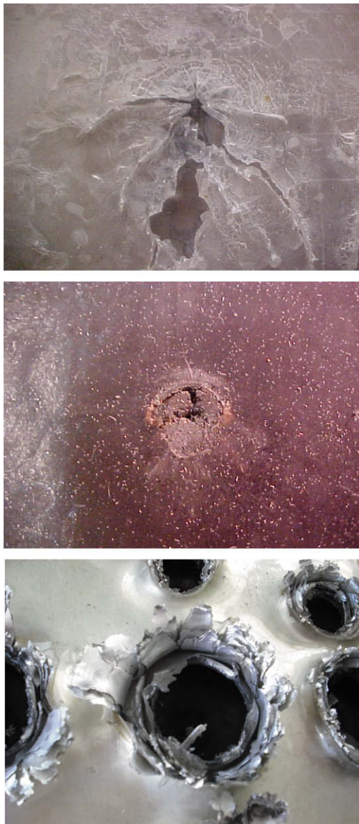
Fig. 2. Upper: Substantial stretching and tearing of low T_g coating that failed in rubbery fashion. Tests with failure modes of this type are indicated by the hollow symbols in Fig. 1. Middle: Brittle failure of high T_g elastomeric coating via shear-dominated separation of a cylindrical section of material having a cross-section matching that the projectile. This failure mode corresponds to the filled symbols in Fig. 1. Bottom: Profuse damage accompanying penetration of HHS coated with 21 alternating soft and hard layers (see Table 4).
