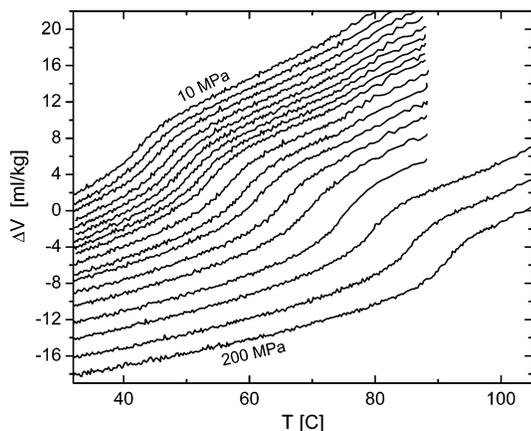
**Figure 2.** Change in specific volume of the terpolymer at (top to bottom) 10, 15, 20, 25, 30, 35, 40, 45, 50, 60, 70, 80, 95, 110, 130, 150, 175, and 200 MPa. The specific volume at ambient temperature and pressure was 0.547 mL/g.
