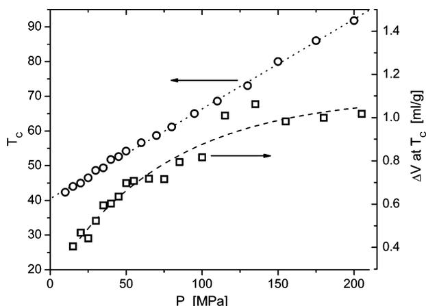
**Figure 3.** Temperature of the Curie transition (○) and volume change at  $T_c$  (□), from the data in Figure 2. The lines through the data are only to guide the eyes.
