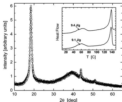
**Figure 6.** Wide-angle X-ray diffraction from the terpolymer. The integral of the crystalline peaks is 38.4% of the total diffracted intensity (neglecting the peaks, at  $2\theta \sim 44^\circ$  and  $51^\circ$ , due to the sample holder). The inset shows the DSC data on the same sample, for which the melting enthalpy measured 20.5 J/g, yielding 53.4 J/g for the perfect heat of fusion.
