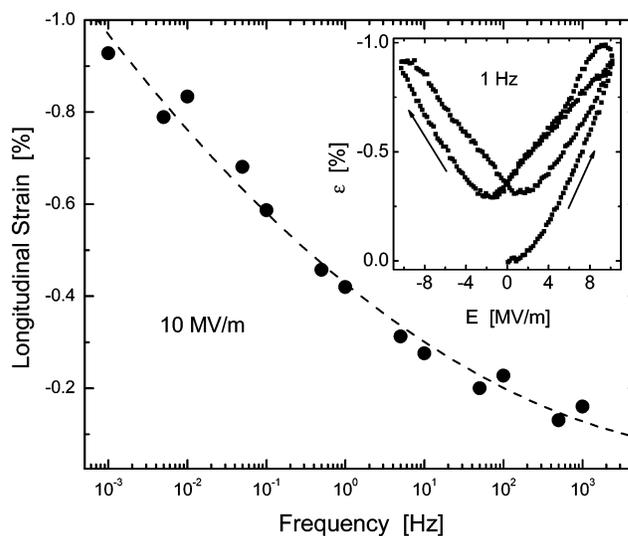
**Figure 1.** Frequency dependence of the thickness (longitudinal) strain in the terpolymer at room temperature. Inset shows the same strain measured as a function of the electric field. There is an offset after the initial cycle, equal to roughly one-third the maximum strain.
