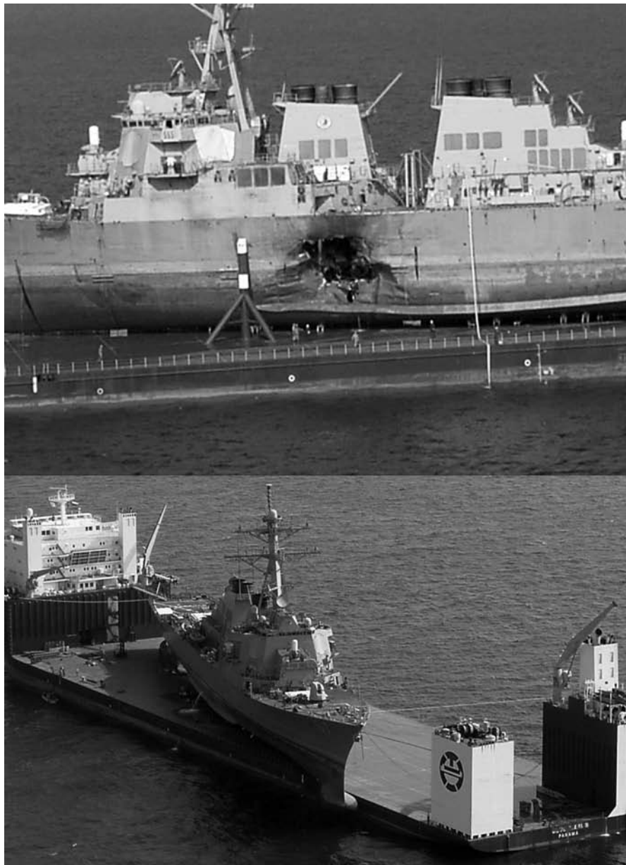
Figure 5.2. The guided missile destroyer USS Cole being returned to the United States after a terrorist attack in Yemen in October 2000. Despite the 150 m 2 gash in the port side of the hull (upper photograph), as well as the jostling when the ship was mounted on a salvage transport vessel, the bow dome (seen in lower photograph hanging off the edge of the transport) was still functional. After repairs that included replacement of 550 tonnes of exterior steel plating, the Cole returned to sea duty 18 months later
