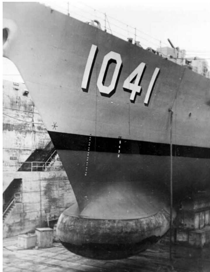
Figure 5.3. Rubber sonar dome assembly mounted to bow of ship
