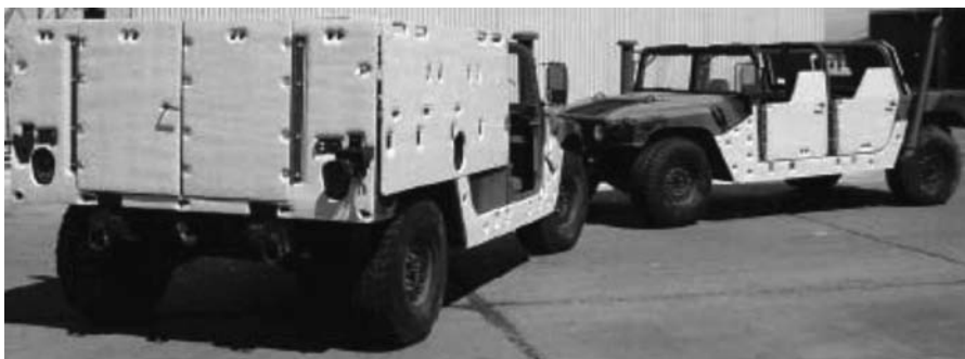
Figure 5.9. Military vehicles with polyurea-coated steel plates on sides of HMMWV and on sides and back of truck
