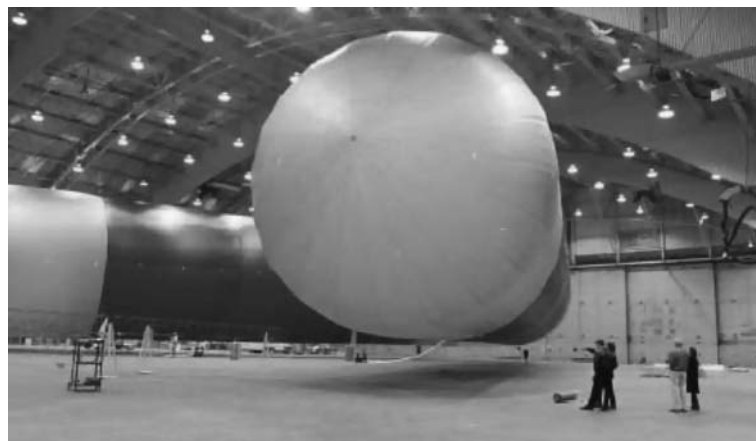
Figure 5.15. Prototype space blimp, 53 m in length, being float tested
