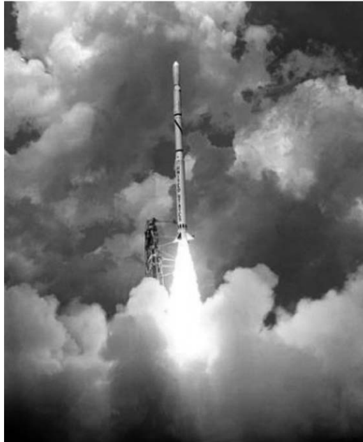
Figure 5.6. Launch of Scout, the only United States' launch vehicle fueled exclusively with solid propellants
