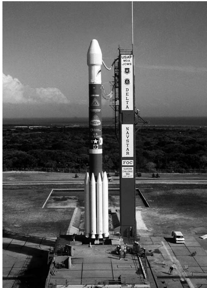
Figure 5.7. Delta III rocket with nine solid rocket motors strapped around the first stage
