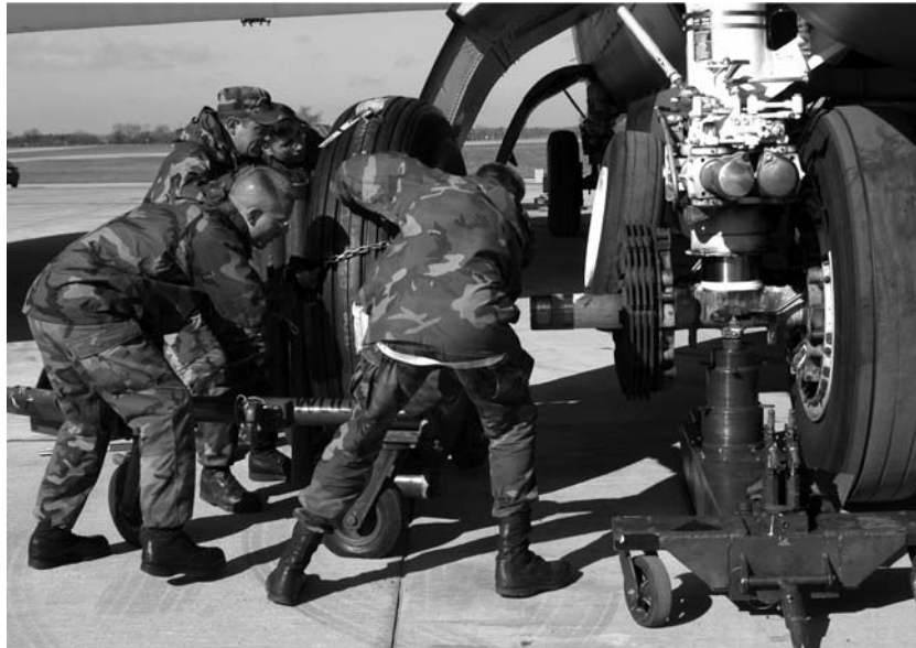
Figure 5.11. Military personnel mount a tyre on a B-52H Stratofortress. The replaced tyre is deflated after its removal. The change-over takes about 20 minutes
