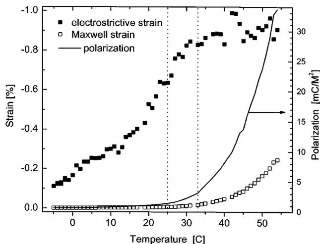
FIG. 1. Longitudinal compressive strain (■) and polarization (—) measured at  $E=10$  MV/m and 0.01 Hz for terpolymer with 7.6% CTFE, along with the calculated Maxwell strain (□). The onset and peak of the Curie transition are denoted by the vertical dotted lines.
