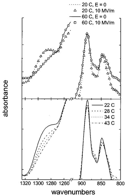
FIG. 3. Infrared spectra of terpolymer (7.6% CTFE) at the indicated temperatures. The Curie transition onsets at 25 °C, with the peak at 33 °C. Lower panel: The sample was heated above the  $T_C$  and allowed to cool slowly back to room temperature, with no electric field present. Upper panel: Two scans below  $T_C$  and two above the  $T_C$ , in each case with and without an applied electric field.
