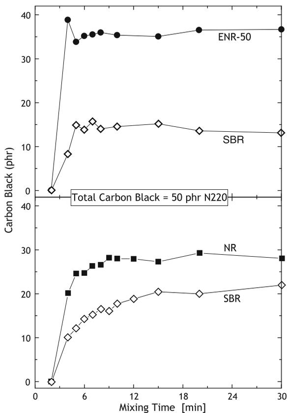
blends are common. This is illustrated in Fig. 12 [85], showing the different uptake of carbon black in blends of SBR with NR, a relatively non-polar polymer, and with a polar, epoxidized natural rubber. The carbon black distribution is more inhomogeneous for the latter.
