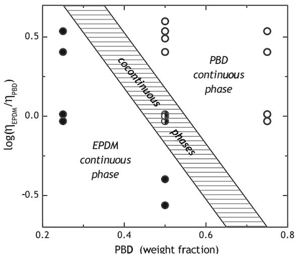
**Fig. 2** Dependence of the phase morphology on the viscosity ratio and composition for blends of PBD and EPDM. Dispersed PBD and EPDM particles are indicated respectively by *open* and *filled symbols*; *half-filled symbols* indicate a co-continuous morphology. Data from Ref. [20]
