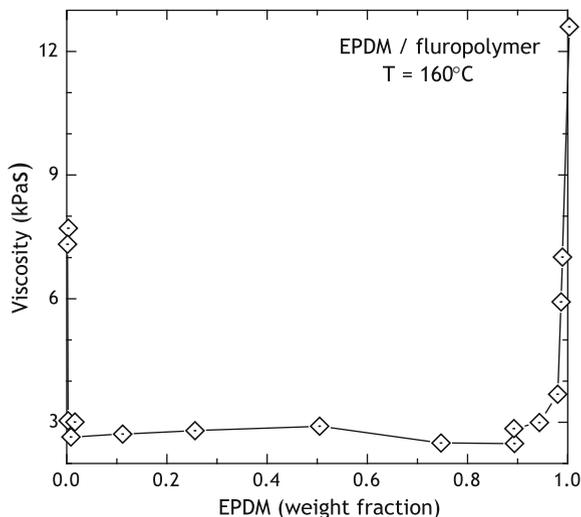
be slippage at the interface. This is seen in the enormous reduction in apparent viscosity in blends of EPDM and a fluoroelastomer (Fig. 10) [66]. The blend exhibits a resistance to flow almost an order of magnitude smaller than for either of the neat components.
