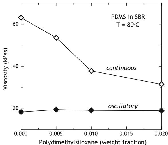
at high concentrations may affect the properties of the cured rubber. An alternative is to add small quantities of a polymeric component of lower viscosity. During processing, the lower viscosity component of a phase-separated blend tends to accumulate at the surface, where the shear rates are largest [61, 62]. The phenomenon of the morphology arranging to accommodate the applied stresses is referred to as the principle of minimum viscous dissipation [63].
